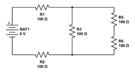
27. What is the equivalent resistance in the circuit?
